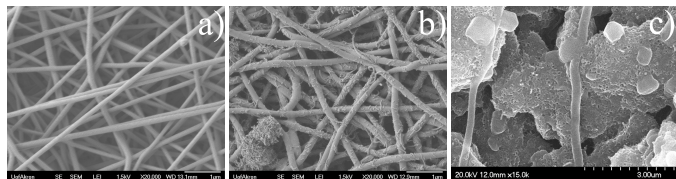
Figure 3. SEM images showing the nanocomposite sensing material. a) neat nylon-6 nanofibers, b) MWCNT functionalized nylon nanofibers, and c) polypyrrole coated composite material.
